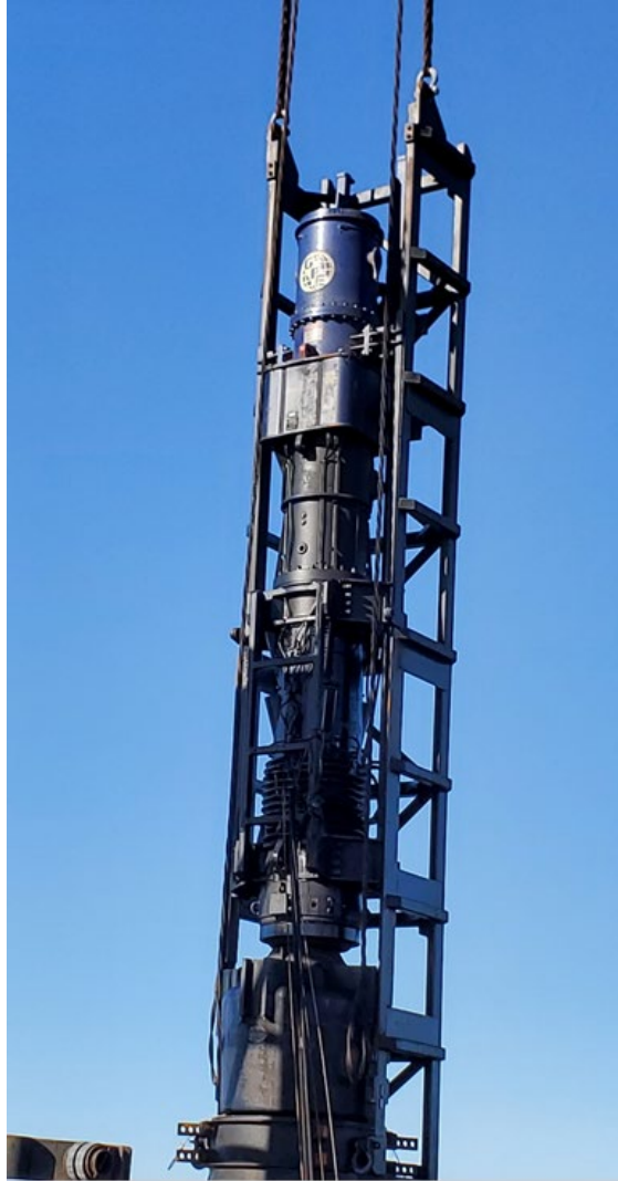
Pileco D180-32 Diesel Hammer; Max. Rated Energy 443.5 kip-ft
